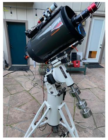
Frank's astrophotography setup, showing, from bottom to top, the white AP1200 tripod and mount with counterweights attached, the large black C14 optical tube assembly with the black Hyperstar unit and red camera attached to its front, and top, the white guide scope and camera attached. (*Frank Seminaro*)
