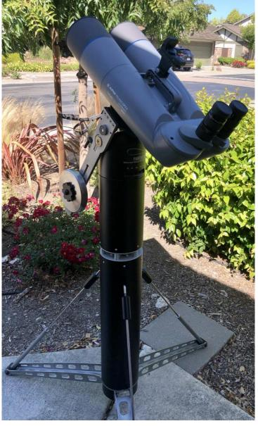
Bill Lockman's APM 100 mm 90 degree apochromatic binocular telescope on top of an altazimuth TTS-160 Panther mount. (*Bill Lockman*)
