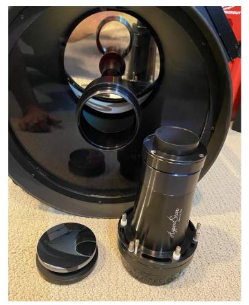
Frank's C14 telescope with its secondary mirror (front left) removed. When attached, the Hyperstar unit (front right) will change the focal ratio of the optical system from f11 to a much faster f2. (*Frank Seminaro*)
