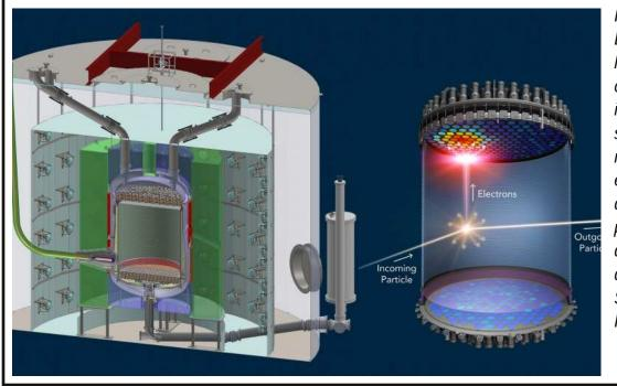
Figure 1. Diagram of the LZ Experiment showing how a possible DM particle could hit a xenon nucleus in the tank causing it to scintillate with light and release a shower of electrons that would be detected by the photomultiplier tubes distributed around the detector. (Courtesy: Sanford Underground Research Facility)
