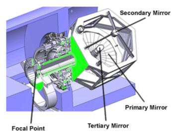
Figure 2 – The SOFIA 2.7-meter IR telescope in its mounting. (*NASA*)
