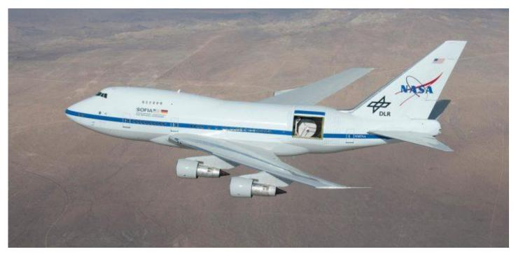
Figure 1 - NASA's SOFIA airborne observatory with telescope visible in the observing portal. (*NASA*)
